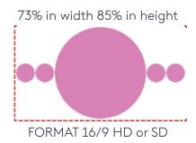
It is therefore necessary to provide a "safe area" of 85% height and 73% width on the 16:9 element (in red on the diagram) to be sure that all the "text and logo" elements of the message will be displayed on all types of screens.
